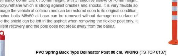
Moulded post with integral shock cord device allows post to revert to upright after impact. Comes complete with sealbrite sleeve, eye on top, black rubber base with 3 holes to screw the fixing bolts. 80 cm height x 100mm Dia.
